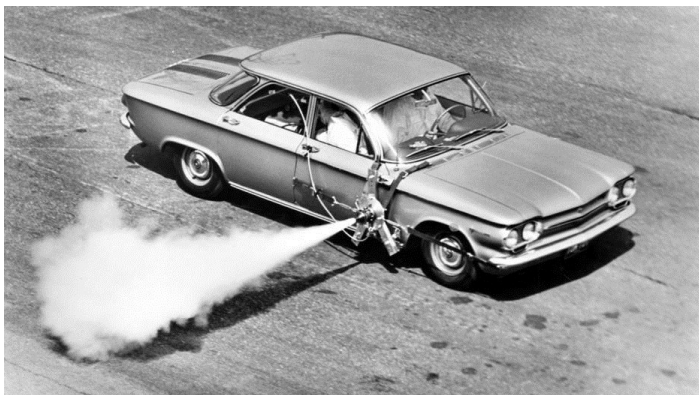
A Sidewinder rocket engine is one way to test stability
