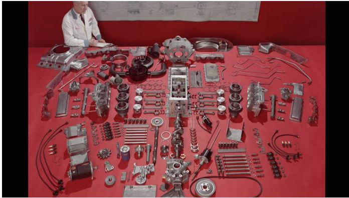
View of a 1960 Corvair flat-six shows the short-stroke crankshaft.
