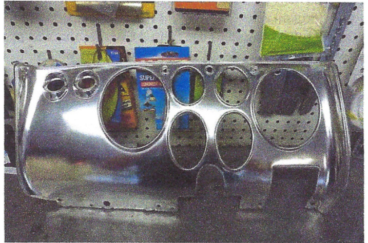
Stripped, Ready for Masking Tape
