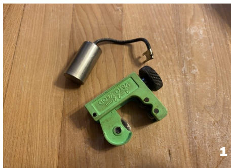
I used a small pipe cutter to trim the cap off the condenser. I was curious to see if there was anything visually wrong inside.
