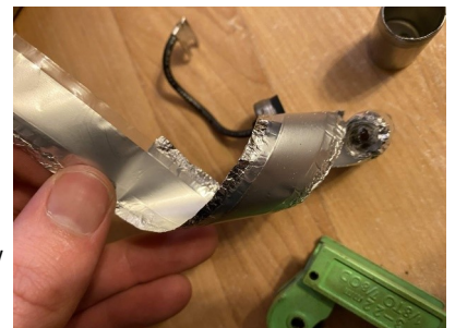
The inside of an ignition condenser is a tightly-wound roll of this foil. This is the material that temporarily holds the charge of the ignition system when the points open.
