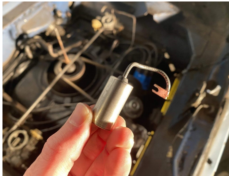
This is the ignition condenser removed from the distributor. It's a humble little piece, but very hardworking.
