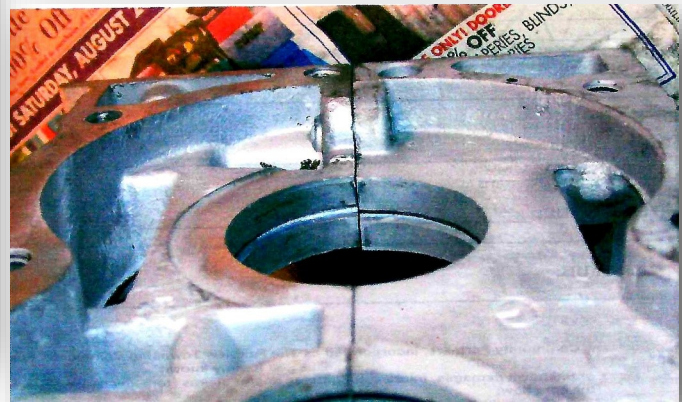
Half Main Drill with 7/32" bit
