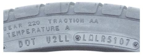
In this example above: DOT U2LL LMLR **5107 51** indicates the 51<sup>st</sup> week of the year in which the tire was manufactured. **07** indicates the year 2007 the tire was manufactured.
