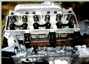
You can see the Push Rod Tubes from the head to block, two for each cylinder.
