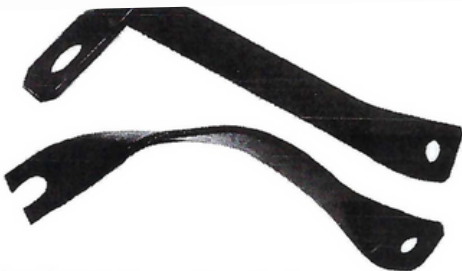
Bend and shape the stock bracket (top) to the shape shown at the bottom.
